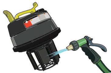
Remove debris from float ball and wire mesh Float Cage housing with hot water.
