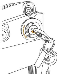
Push key IN and rotate counter clockwise to Unlock.
