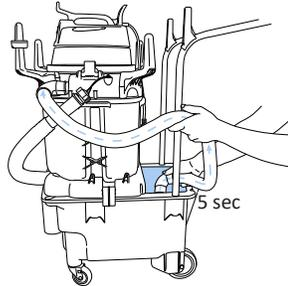
Alternatively, you can also turn Vacuum on and dispense solution into Vacuum Hose as shown to clean Hose and Tank.
