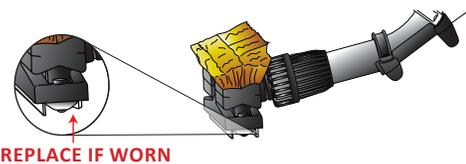
Check for worn squeegee blades. Worn blades cause streaking and loss of vacuum suction.
