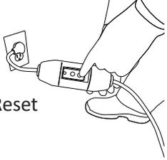
A line drawing showing a hand pressing the "Reset" button on a GFCI outlet. The word "Reset" is written below the button. |
