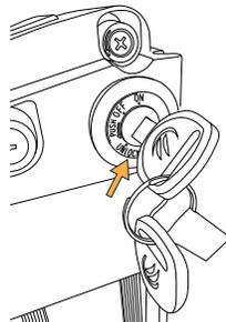
Key needs to be in unlock position to remove.
