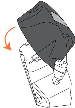
Connect the plug from the battery housing into the vacuum motor plug.
