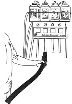
Rinse Vacuum Tank thoroughly at clean-up sink, preferably with hot water. Rinse out Trolley Bucket. Rinse foam filter inside Vacuum Tank and Trolley Bucket. Rinse plastic finger filter in both components following to clear debris. Clean the mixing solution assembly and orifice.
