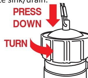
Once cap is removed, lower Dump Hose into appropriate sink/drain. To prevent an accidental spill or overflow from the Dump Hose, be careful to keep hose end upright until it is over sink/drain.
