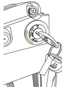
Once in place, turn key clockwise to OFF to lock in place.
