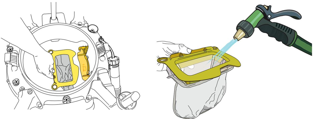
Before starting each recycle process, remove Filter Bag, dump any debris out, spray clean, and replace.
